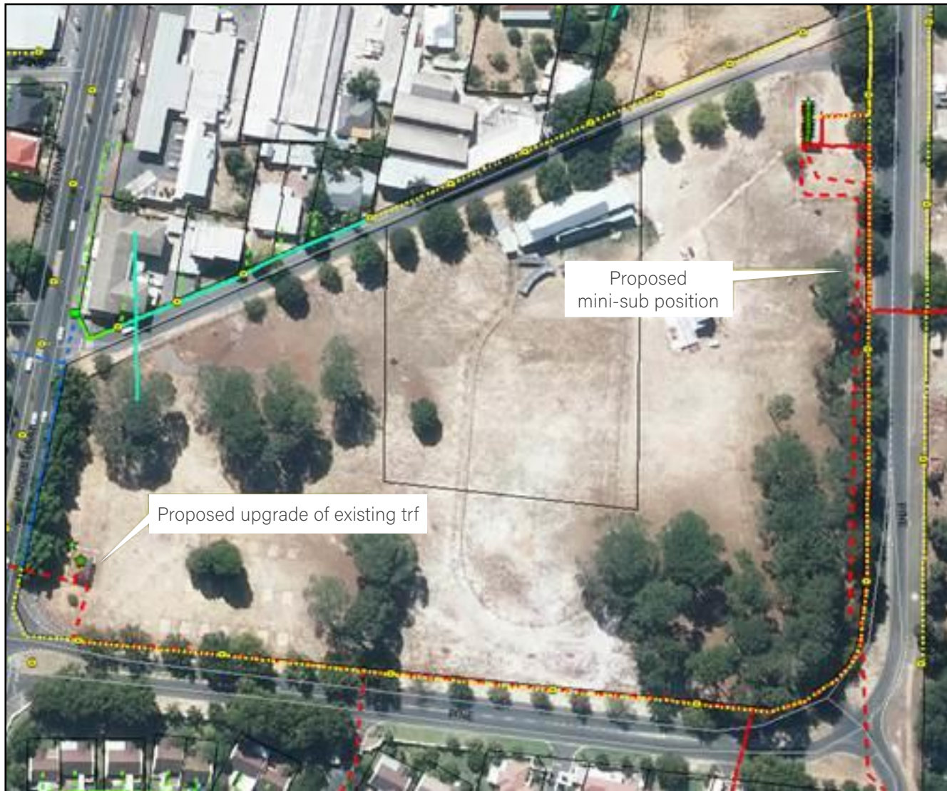
Figure 65: Schematic illustrating location of proposed mini-substation and the upgrading of the existing transformer
