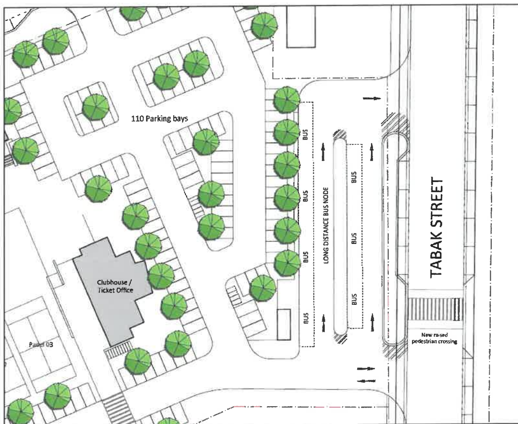
Figure 41: Bus Parking Area
