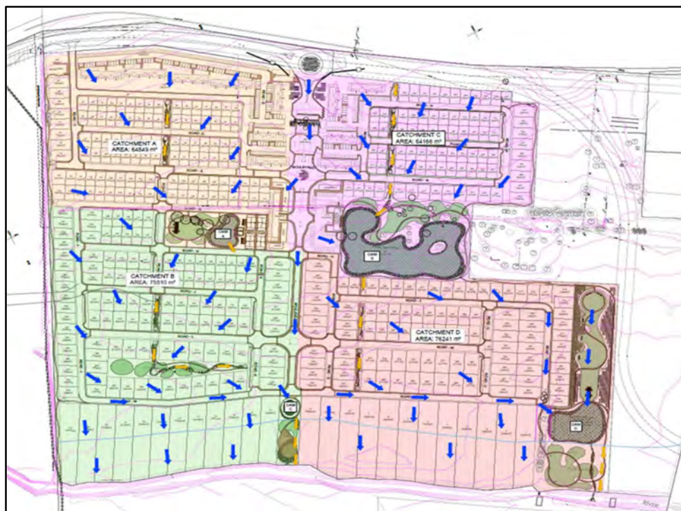
Figure 19: Overland Drainage Patterns and Attenuation facilities
