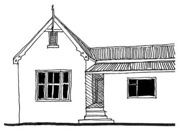
Removal of key elements (timber/cast-iron columns) and replacement with unsympathetic and inappropriate materials (square face brick columns).
