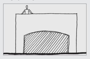
The roof deck/terrace on top of the garage is inappropriate because it creates extreme wall heights.
