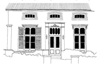
Building too wide for a single roof, resulting in either out-of-scale buildings or squat proportions. Gable window too large – should be same/smaller than ground floor windows.
