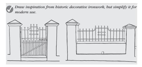
Use simple plaster mouldings to decorate the gate pillars and walls of the entrance gate, while the steelwork is more ornate.
