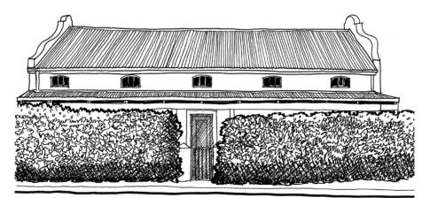
Permeable fencing on top of a base of brickwork is a good security solution reducing the visual impact of wall height, while maintaining a connection between house and street.
