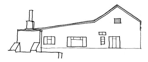
The original doors have been removed and replaced with standard catalogue doors that are narrower and shorter.
